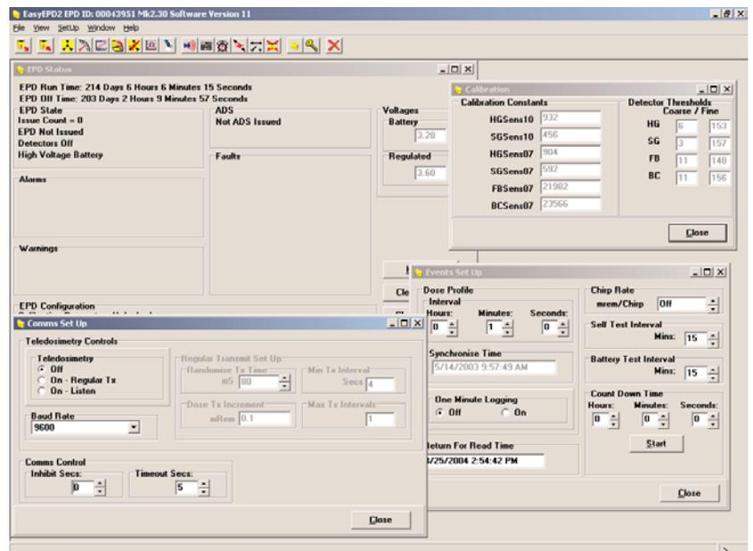
EasyEPD2 may be used for simple issue and return of dosimeters, with read/write logging of data. It also provides secure access to all dosimeter functions, offering the ability to set all parameters and carry out maintenance and diagnostic work.
