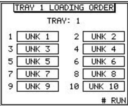
Keep it simple. Can you just walk up to the instrument and run a generic wipe? Absolutely! That is why we pre-programmed GENERAL into the Library. Choose General, and run a wipe test. The counter reads in a wide window and identifies any isotope windows which exceed the preset trigger. The results are recorded as wipe#1, wipe#2, etc. Nothing to pre-program-just count and report.
